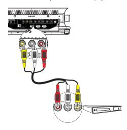
You can also connect the supplied AV switch cable to the AV FRONT jack first, then connect the AV cable to the AV output jacks on the DVD player.
